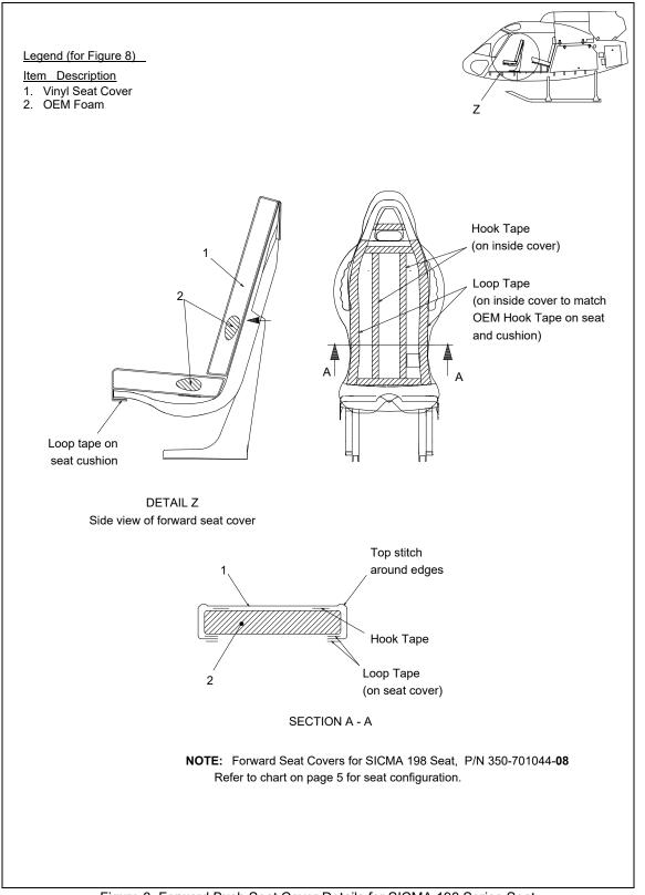
Figure 8 Forward Bush Seat Cover Details for SICMA 198 Series Seat
