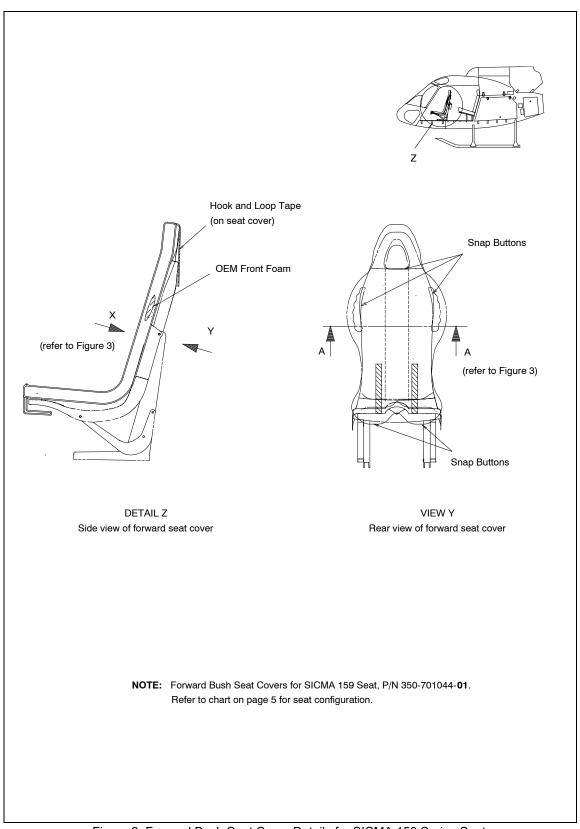
Figure 2 Forward Bush Seat Cover Details for SICMA 159 Series Seat
